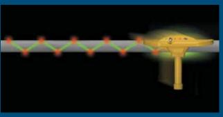
With the AML parallel with the pipe or underground object, you can now scan the entire length of the object's edge. As an alternative, utilize the "W" method of scanning by sweeping the area in a back-and-forth "W" motion, marking the object's location and run direction as it is tracked.
