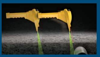
Holding the AML's handle parallel to the ground, scan the area of the undetectable buried object until one or both of the target indicators activate.
